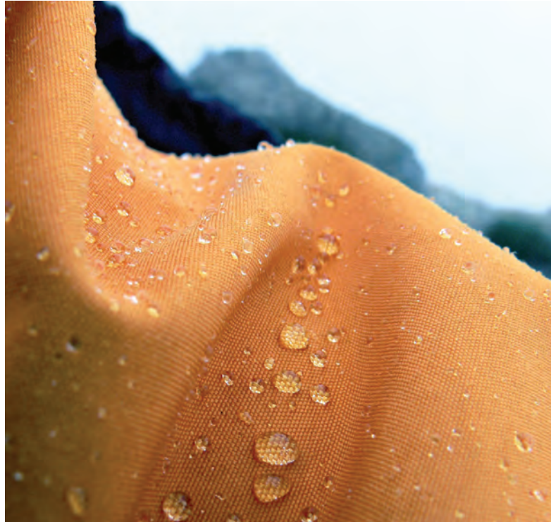
By transforming ePTFE into a thin, porous membrane, Bill and Bob Gore were able to create a new material that was waterproof and breathable at the same time. Photo: Manuel
