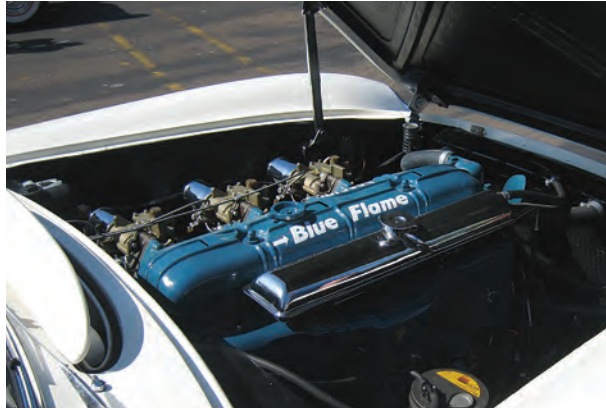
The car's six-cylinder "Blue Flame" engine Photo: Kowloonese
