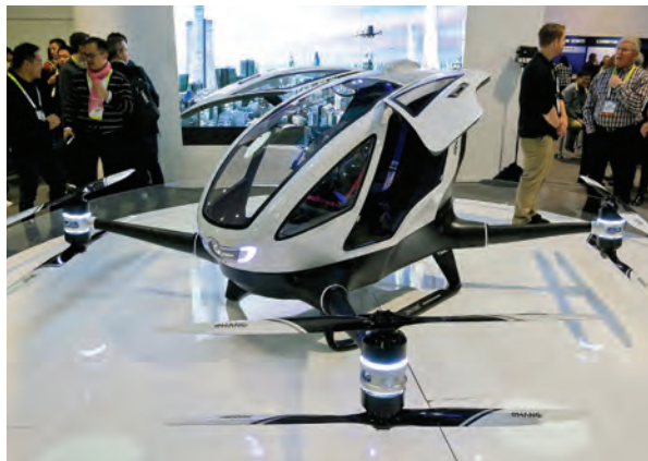
Chinese company EHANG has built a prototype quadcopter capable of carrying passengers.
