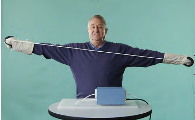
Bob Gore demonstrates how quickly stretching a rod of PTFE led to his accidental discovery.
